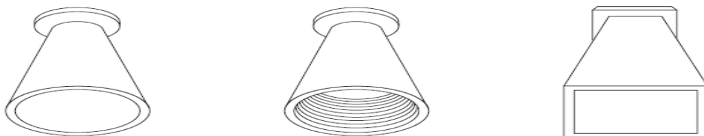
Figure 6.10 Horn antennas: (a) smooth-walled conical, (b) corrugated, and (c) pyramidal.
